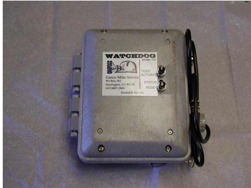
This voice enunciator is designed to allow the operator to record a 15-second message for broadcasting over a standard pager telephone system. The message can alert personnel of status changes in the monitored piece of equipment. Another feature permits monitoring of heat detection sensor cable. The belt heat detection and notification of open, short, and fire required by CFR 30 are included.
